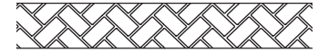
HERRINGBONE HEADER BRICK SIZE: 3 \frac{3}{8}'' \times 7 \frac{5}{16}'' ROLL WIDTH: 8 \frac{9}{16}'' JOINT WIDTH: \frac{1}{2}''
