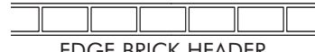
EDGE BRICK HEADER BRICK SIZE: 4 \frac{1}{8}'' \times 8 \frac{15}{16}'' ROLL WIDTH: 5 \frac{1}{8}'' JOINT WIDTH: \frac{1}{2}''
